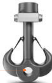
RAMSHORN FORM B (Drop Forged, Machined with Crosshead, Nut and Latches)
