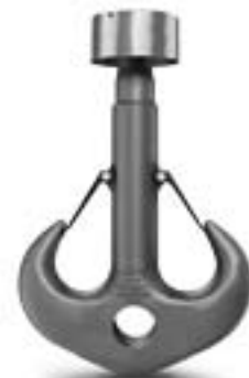
RAMSHORN FORM B (Open Die Forged, Machined with Nut and Latches)
