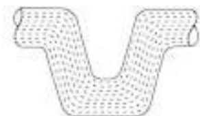
FORGING Uniform grain flow gives material higher strength
